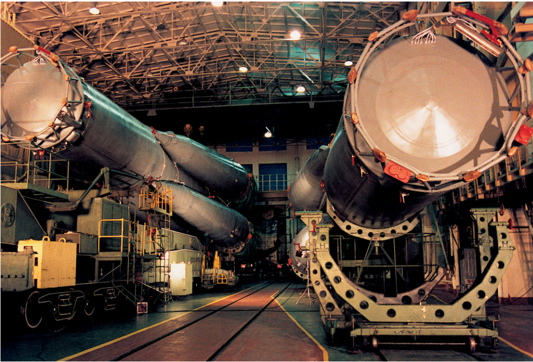
Figure 2-3. Two Soyuz-U boosters (first and second stages only) in the MIK integration hall in Plesetsk, 27 December 1992. The launcher is assembled and rolled-out horizontally while lying on a railway wagon shown left. Rotation into the vertical position takes place at the launch pad. (Photo: L. Pieroni)
