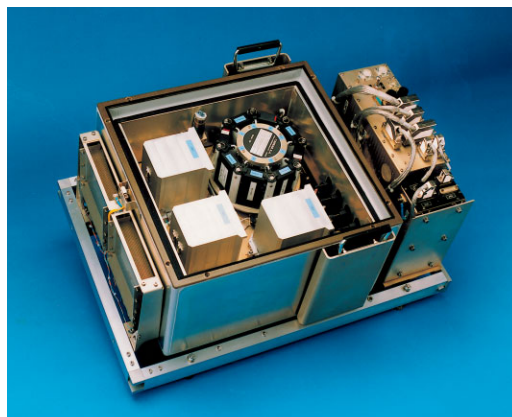
Figure 6-5. Biobox, with the lid removed, factory-fresh in June 1992. The three CIS containers and the centrifuge were mounted on a platform inside the incubator box. The picture shows Biobox on its handling frame, the two hand-grips fitted to a rectangular support structure. The handling frame was removed before flight. Photo: Dornier.
