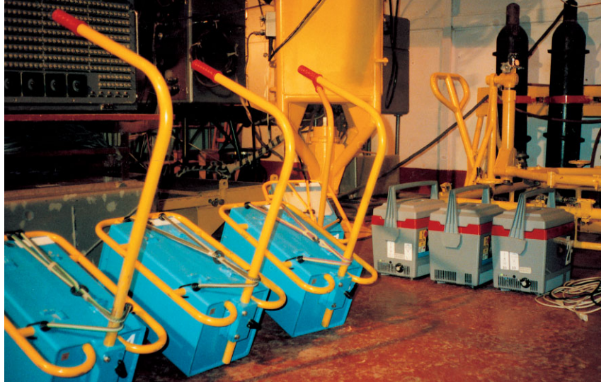
Figure 3-7. Trolleys and thermal boxes in the MIK. The autonomous experiments were transported from Moscow to Plesétsk in thermal boxes (shown right). During transportation the boxes were carried on trolleys (shown left) and were powered by batteries contained inside the blue packing cases.
