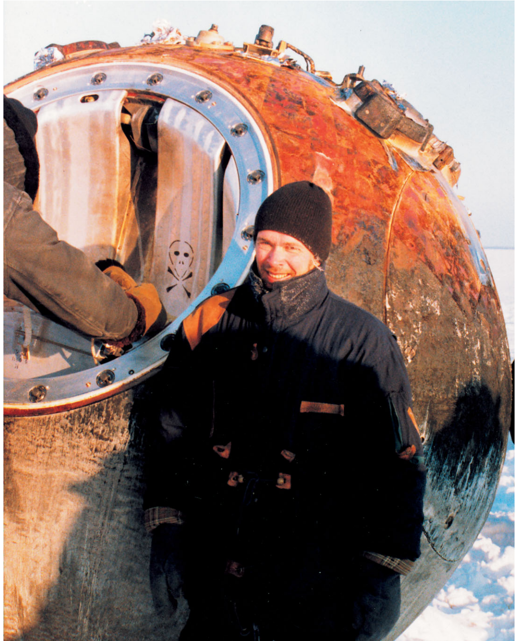
Figure 3-12. A Bion capsule after landing. The photograph shows Bion-11, which was very similar to Bion-10. Note the KNA containers on top of the capsule and the open parachute hatch. (Photo provided by Yu. Evstratov).
